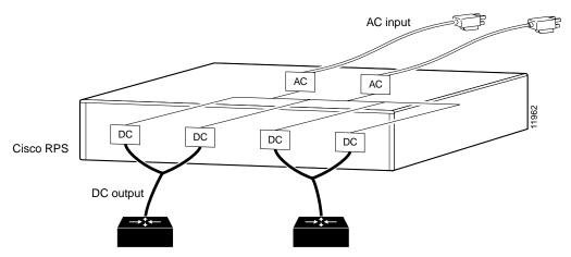
Figure 8 Redundant-with-Reboot Configuration
